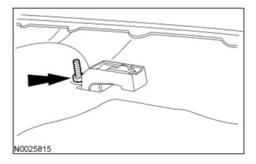
3. **NOTE:** Push upward on the exterior door handle actuating rod and make sure the door latch is in a neutral position when installing the rod into the retaining clip to make sure the exterior door handle is correctly positioned.
