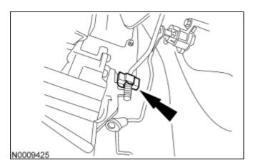
5. **NOTE:** Two exterior door handle studs must be removed on the RH side.
